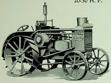
Will pull three 14-inch moldboard plows under average conditions and a proportionate number of disc plows. It will handle up to a 28-inch thresher fully equipped, or a medium sized silo filler or corn shredder
