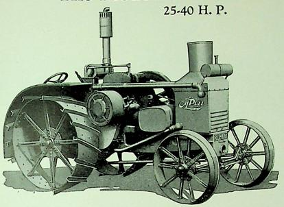
Will pull four 14-inch plows under average conditions and handle up to a 32 x 52 Rumely thresher and up to a 10-foot road grader
